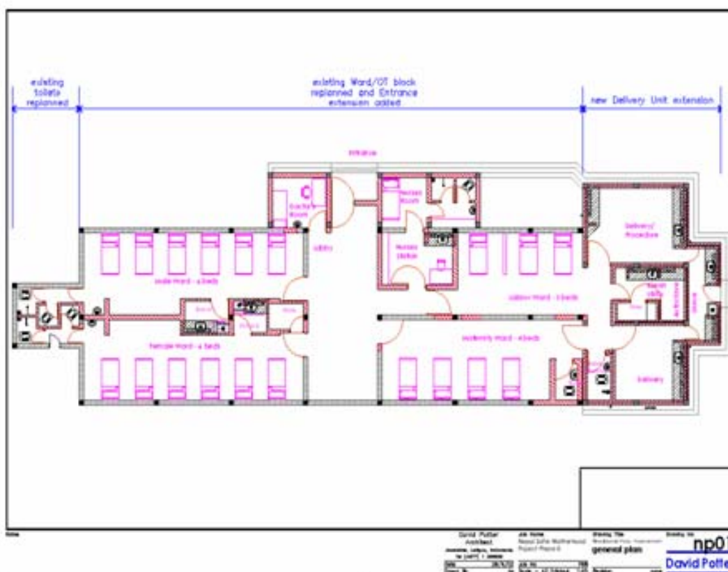
Proposed architectural plan for new extension of delivery suite, internal alterations of building and link passage to emergency/out-patient unit
